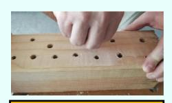
6. Gently sand the nesting holes. Splinters can remain after drilling, but removing splinters will make the nesting box more appealing for bees.
