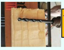
4. Check the depth of the holes, which should be about the length of most drill bits.
